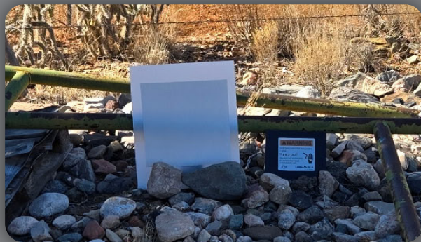
Left: White field sample | Right: Warning graphic sample Positioned during daylight hours at the far end of the MIGS property for long-range visibility testing.
